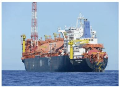
This activity included also side-by-side mooring/unmooring, loading arms connection, gassing-up of all cargo tanks, cooldown of all cargo tanks and LNG cargo offloading of a volume of 109.000 cubic meters. The liquefied natural gas in this phase is a clear liquid devoid of any smell. The process of odorization occurs only when the gas is injected into the network in function of its use for various typologies of users.
